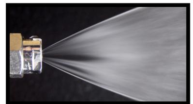
The **flooding (flat fan)** nozzle delivers a wide angle flat spray pattern. It operates at very low pressure and produces large spray droplets. Its pattern is fairly uniform across its width but not as even as the regular flat fan nozzle pattern. If used for broadcast spraying, it should be overlapped to provide double coverage. It is often used for applying liquid fertilizers or fertilizer/pesticide mixtures.
