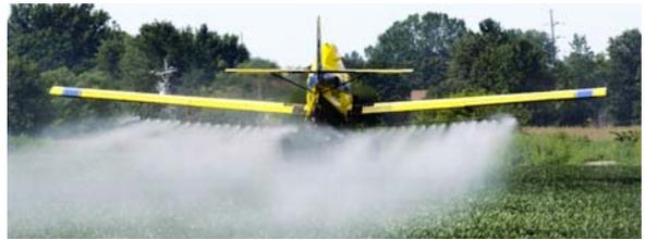
by measuring how much water is used during several test flights. Each time you fill the tank you will make a run operating the sprayer for a timed period.
