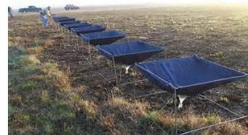
Fly a swath test along a centerline oriented at a right angle to the line of collection pans. If ambient wind speed is greater than a sustained 8 mph, orient the line of pans at a right angle to the prevailing wind and fly directly into the wind.
