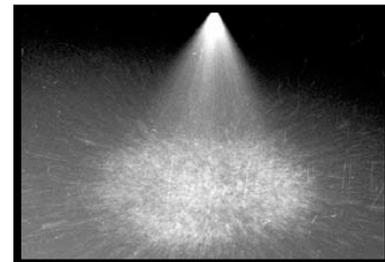
**Core-insert cone** nozzles produce either a solid or hollow cone spray pattern. They operate at moderate pressures and give a finely atomized spray. They should not be used for wettable powders because their small passages clog easily and they wear rapidly due to abrasion.
